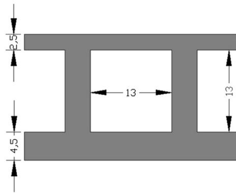
Fig. 6. Cross sectional view of the first wall (mm).
