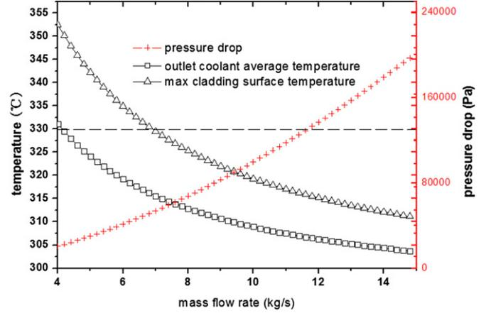
Fig. 13. Values of temperature versus mass flow rate.
