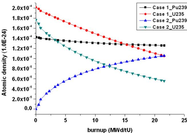
Fig. 12. Atomic densities of the fissile isotopes as a function of burnup.
