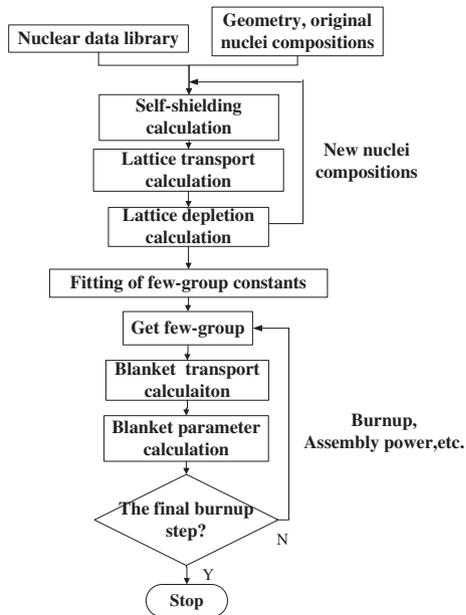
Fig. 5. Computational flow chart of neutronics code system.
