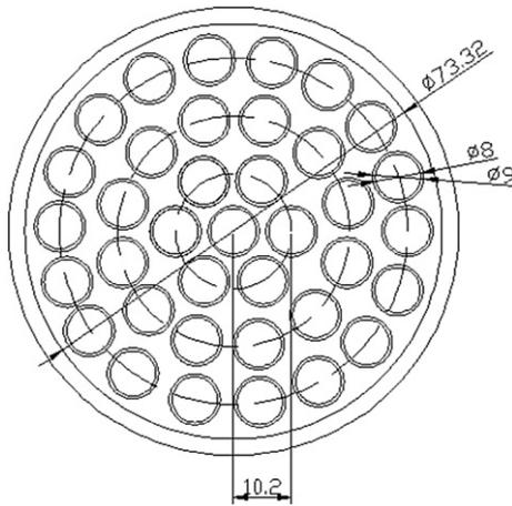
Fig. 4. Cross sectional view of the outer blanket (mm).
