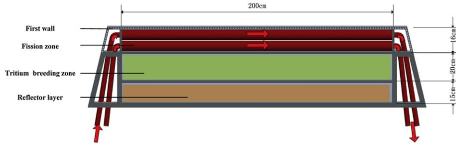
Fig. 3. Cross-section of outboard.
