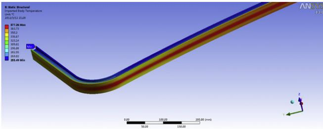
Fig. 8. Temperature distribution in the first wall.
