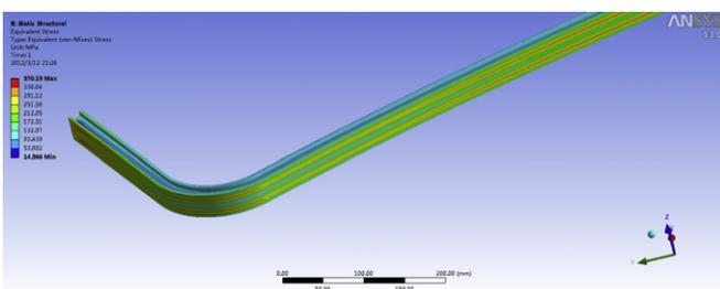
Fig. 9. Thermal stress distribution in the first wall.
