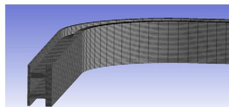
Fig. 7. Mesh of the first wall.
